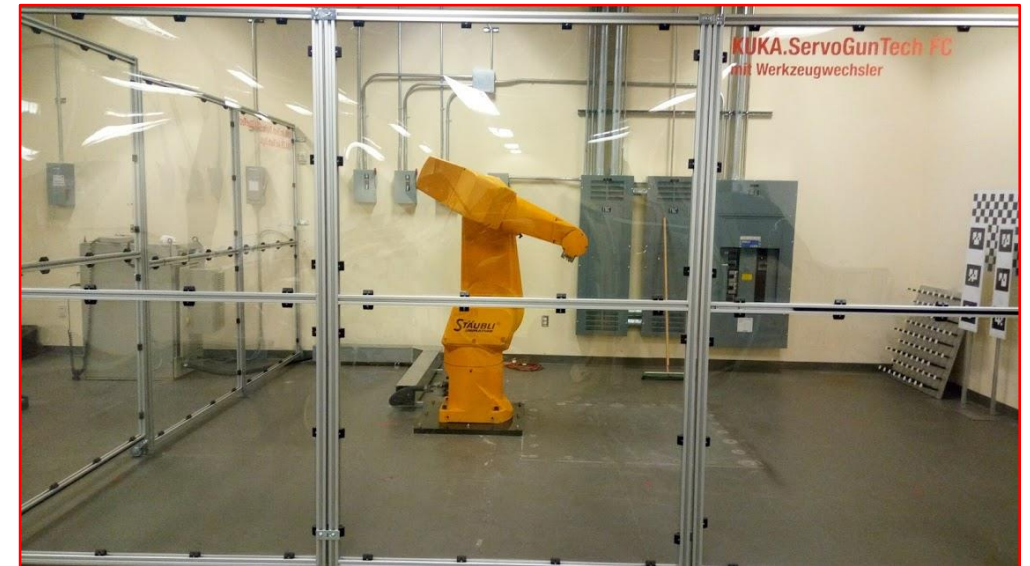
Robotic grinding testbed under construction at IRIM Techway Robotics Lab
